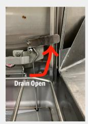
**CLEANING:** Push the OFF button. Raise the door. Drain the machine by lifting the drain lever. Remove and clean out the strainer bucket and pan.
